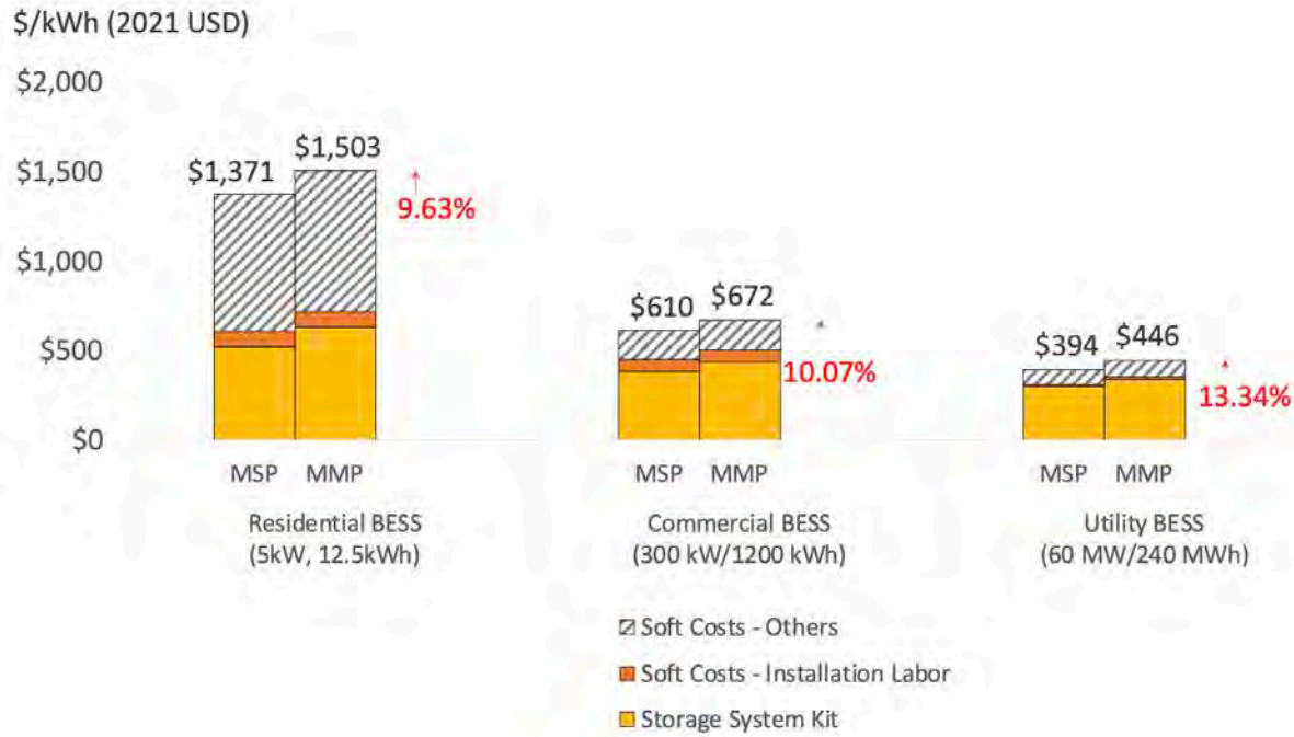
Figure ES-2. Q1 2022 U.S. standalone battery energy storage system (BESS) cost benchmarks
